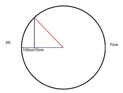
We can see in this illustration of a two meter drive above that upon deflection the radius for calculating centripetal acceleration having rotated from a..b (Aft) becomes a radius of 70cm versus 100cm using a two meter drive template.
